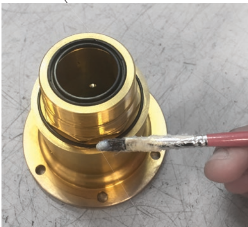
Apply a coat of grease to O-ring
