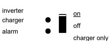
The AC input voltage is switched through and the charger is switched off.
