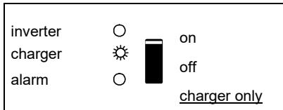
The AC input voltage is switched through and the charger operates in float mode.
