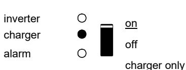
The AC input voltage is switched through and the charger operates in bulk or absorption mode.
